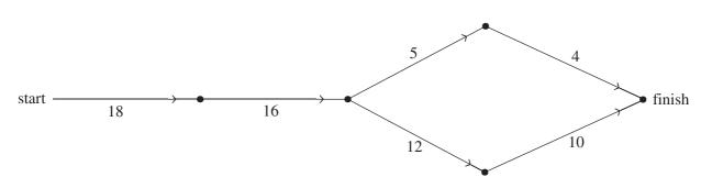
Using the 'minimum-cut, maximum-flow' theorem, the maximum flow through the above network is
